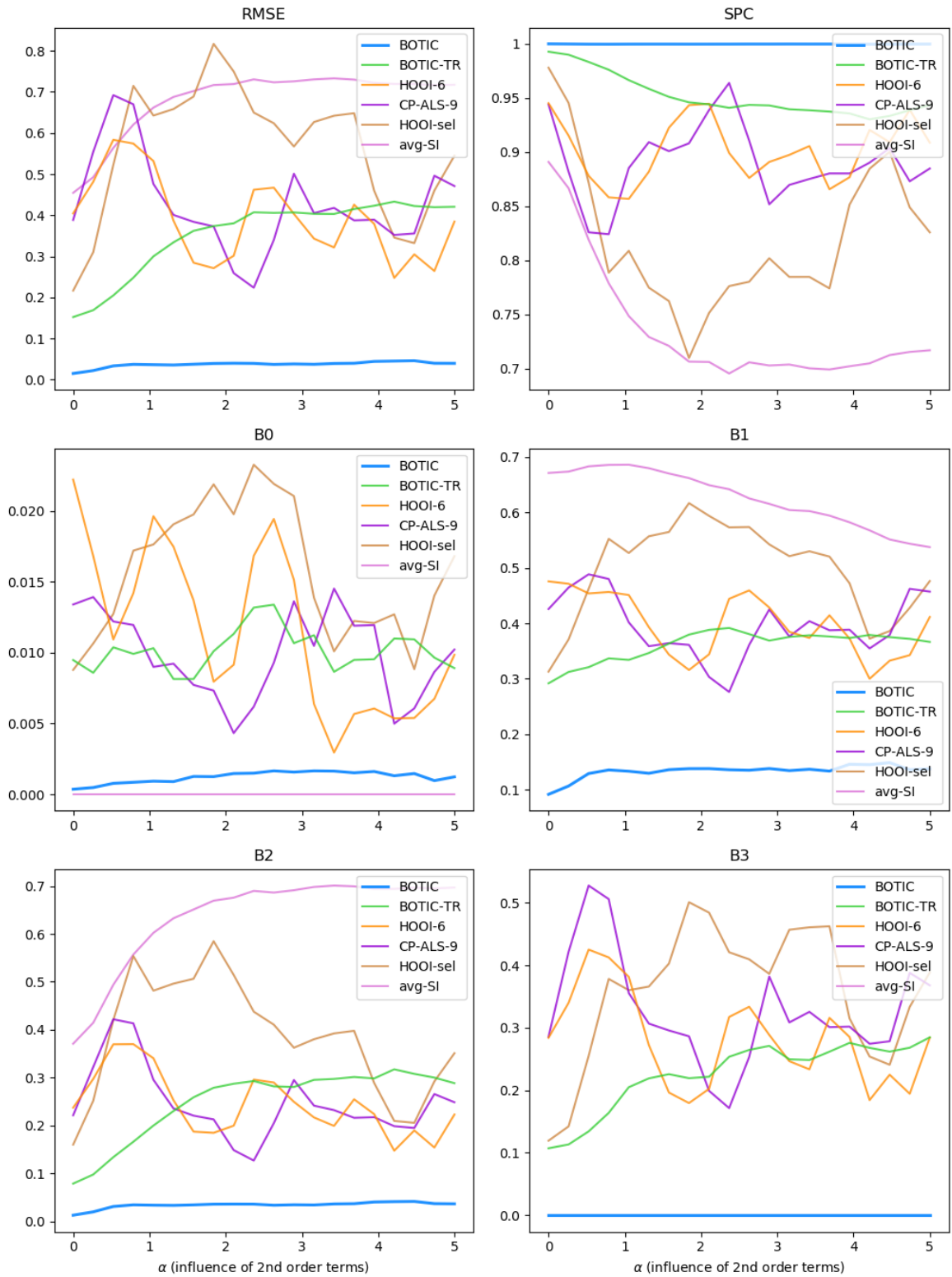
Figure 6: A selection of methods under an increasing relevance of second order terms, p=5\% . Note that optTR is excluded due to poor performance and avg-SI has a consistent B3 of zero.
